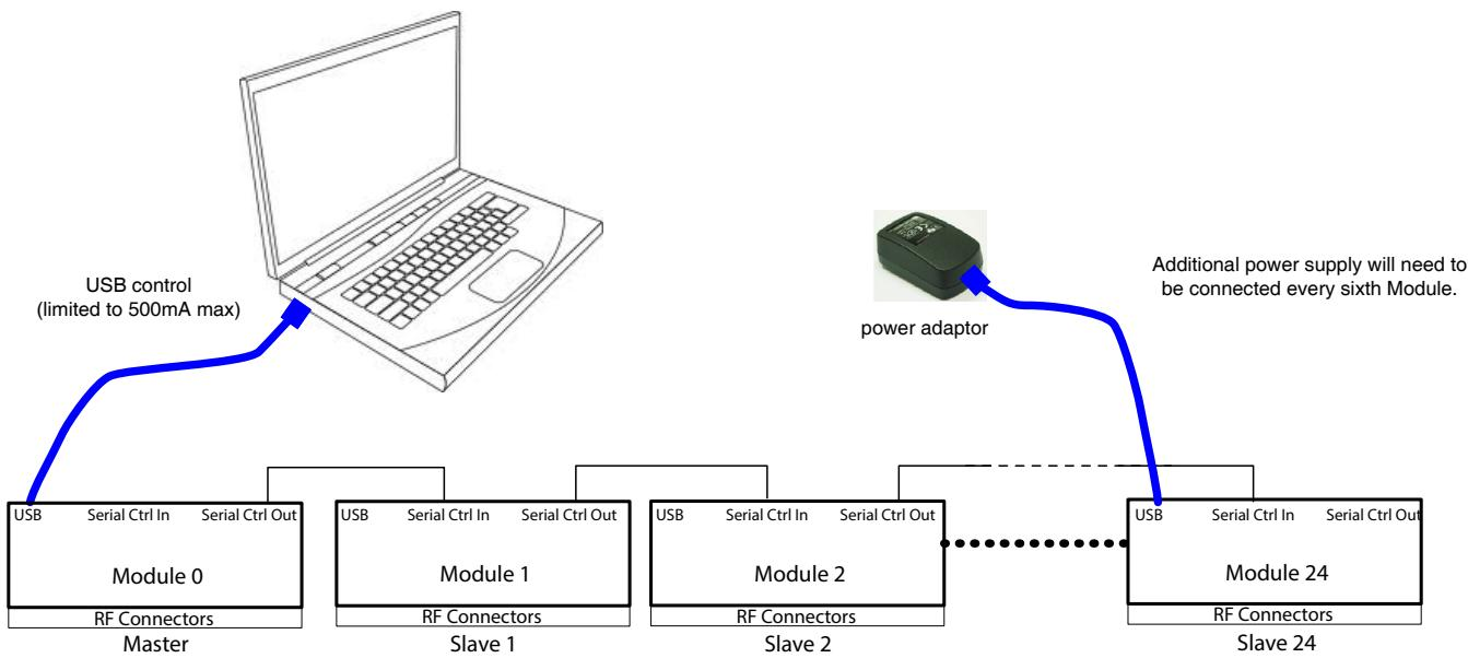
Connections between modules will be made using the serial in/out ports with the module connected to the PC act as a master and all other as slave modules. All control will be through the master module (address 0) which is the only one communicating with the PC. Serial control out port of each module should be connected to the serial control in port of the next module.
