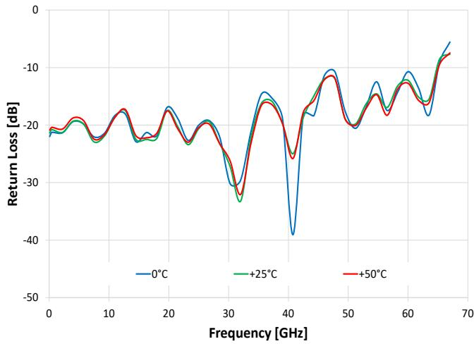
Return Loss @ RF2 over Temperature (RF2 Terminated)
