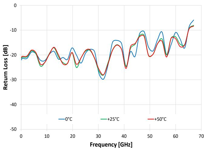
Return Loss @ RF1 over Temperature (RF1 Terminated)
