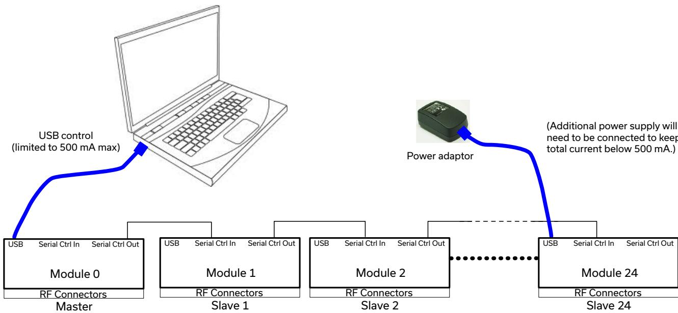
Connections between modules will be made using the serial in/out ports with the module connected to the PC act as a master and all other as slave modules. All control will be through the master module (address 0) which is the only one communicating with the PC. Serial control out port of each module should be connected to the serial control in port of the next module.
