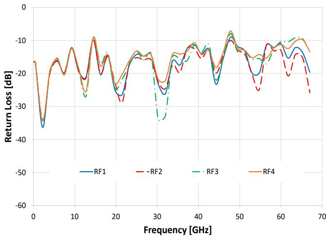
Return Loss @ Terminated ports (RF1 - RF4 Terminated)
