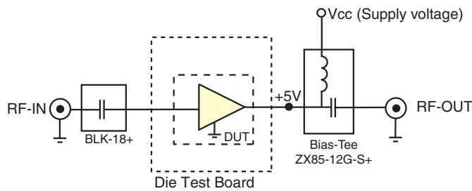
Fig 1. Block Diagram of Test Circuit used for characterization.
