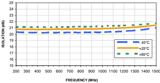
**ISOLATION vs. FREQUENCY & DEVICE VOLTAGE**
