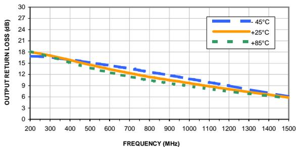
**OUTPUT RETURN LOSS vs. FREQUENCY & DEVICE VOLTAGE**
