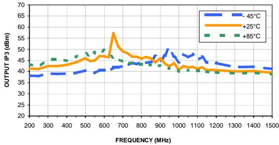
**OUTPUT IP3 vs. FREQUENCY & DEVICE VOLTAGE**
