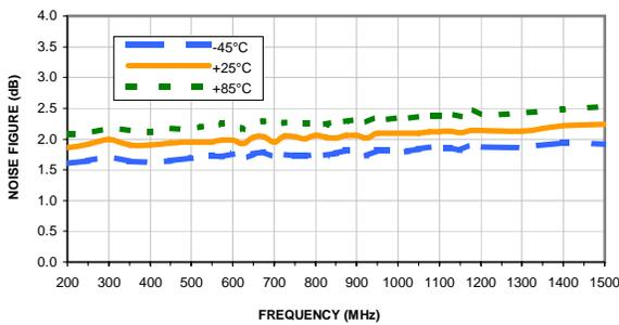
**NOISE FIGURE vs. FREQUENCY & DEVICE VOLTAGE**
