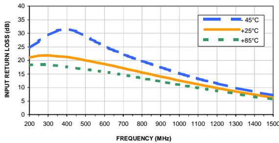
**INPUT RETURN LOSS vs. FREQUENCY & DEVICE VOLTAGE**
