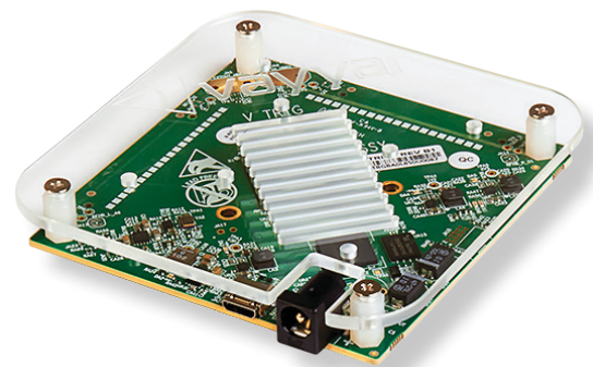
Fig. 1 IMAGEVK-74 RF Sensor
