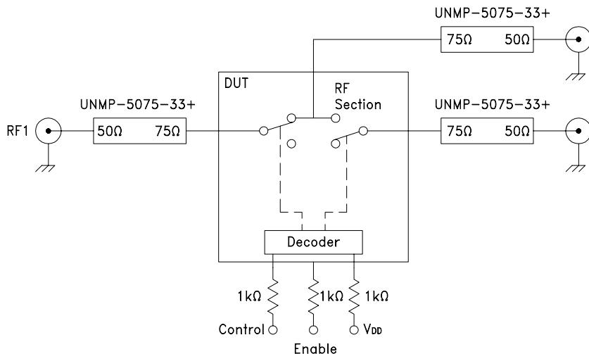
Figure 1: Block Diagram Of Test Circuit Used For Characterization.
