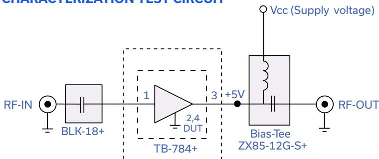
Fig 1. Block Diagram of Test Circuit used for characterization. (DUT soldered on Mini-Circuits Characterization test board TB-784+) Gain, Return loss, Output power at 1dB compression (P1 dB), output IP3 (OIP3) and noise figure measured using Agilent's N5242A PNA-X microwave network analyzer.
