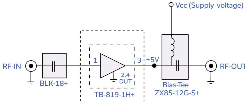
Fig 1. Block Diagram of Test Circuit used for characterization. (DUT soldered on Mini-Circuits Characterization test board TB-819-1H+) Gain, Return loss, Output power at 1dB compression ( $P_{1\text{ dB}}$ ), output IP3 (OIP3) and noise figure measured using Agilent's N5242A PNA-X microwave network analyzer.
