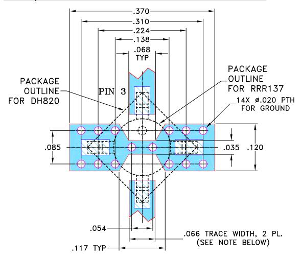
NOTE: 1. TRACE WIDTH IS SHOWN FOR ROGERS RO4350B WITH DIELECTRIC THICKNESS .030"  $\pm$  .002"; COPPER: 1/2 OZ. EACH SIDE. FOR OTHER MATERIALS TRACE WIDTH MAY NEED TO BE MODIFIED.
