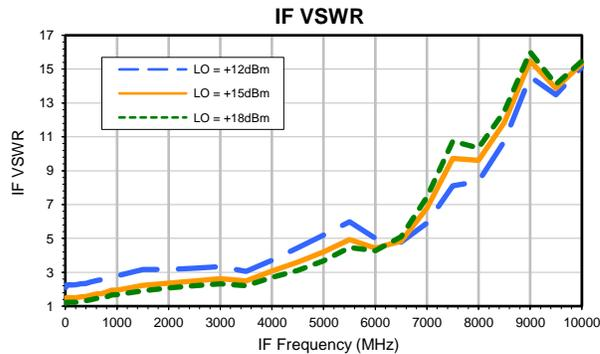
Note: Test data measured in industry standard 4x4mm, 24-lead package
