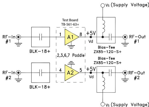
**Fig 1a.** Block Diagram of Test Circuit used for characterization. (DUT tested in Mini-Circuits Test board TB-561-63+, except for IP2). Gain, Return loss, Output Power at 1dB compression (P1 dB), output IP3 (OIP3) and noise figure measured using Agilent's N5242A PNA-X microwave network analyzer.
