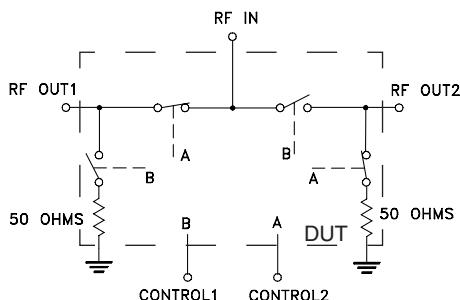
**Figure 1.** Block Diagram of test Circuit used for characterization
