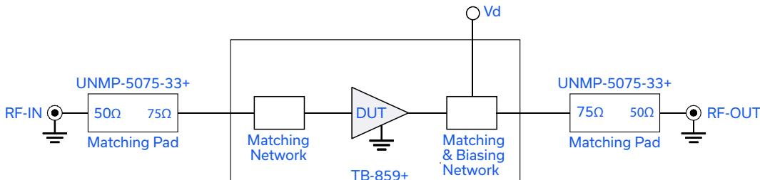
Fig 1. Block Diagram of Test Circuit used for characterization. (DUT tested on Mini-Circuits Characterization Eval board TB-859+)
