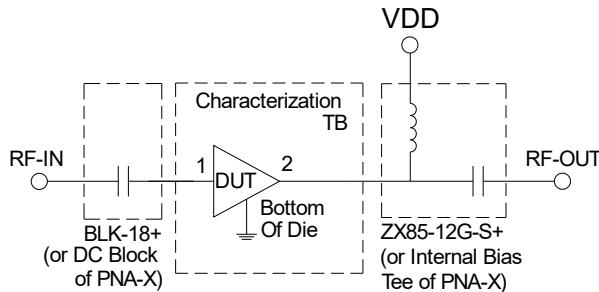
**Fig 1A. Block Diagram of Test Circuit used for S-Parameter and Noise Figure Measurement. (DUT is packaged in SOT-89 and soldered on Mini-Circuits Characterization test board.) Gain, Return loss and noise figure are measured using Agilent's N5242A PNA-X microwave network analyzer.**
