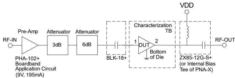
**Fig 1B. Block Diagram of Test Circuit used for P1dB Measurement. (DUT is packaged in SOT-89 and soldered on Mini-Circuits Characterization test board.) Output power at 1dB compression is measured using Agilent's N5242A PNA-X microwave network analyzer.**
