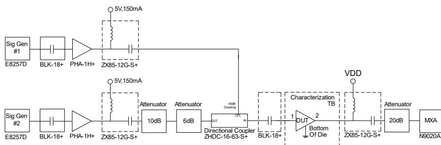
**Fig 1C. Block Diagram of Test Circuit used for IP3 Measurement. (DUT is packaged in SOT-89 and soldered on Mini-Circuits Characterization test board) P1dB is measured using two E8257D Signal Generators and one N9020A MXA Signal Analyzer.**
