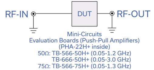
Fig 1b. Block Diagram of Test Set up used for characterization of Gain, IP2, IP3. Measured using Agilent's signal generators E8527D and Spectrum analyzer N9020A.
