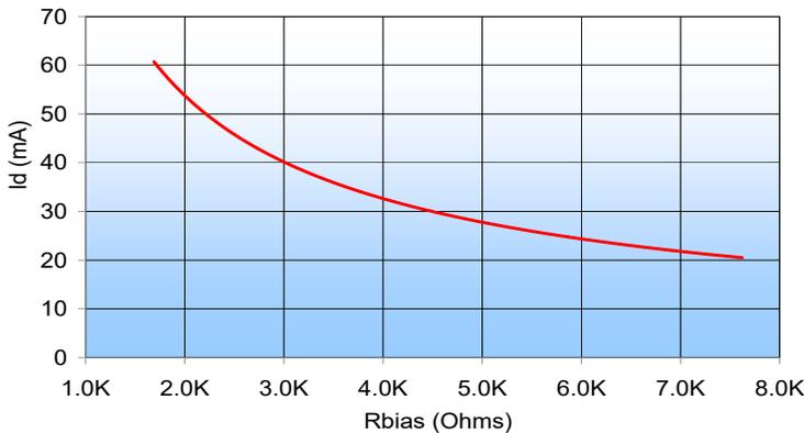
Fig 4.  $I_d$  varies as a function of  $R_{bias}$ . The  $I_d$  current range is defined based upon the specific  $R_{bias}$  value noted in the Application Circuit (Fig 3).  $R_{bias}$  may be adjusted to optimize  $I_d$  for a customers' application. RF performance will vary accordingly.
