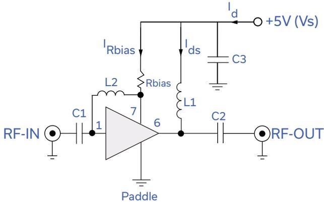
Fig 3. Recommended Application Circuit
