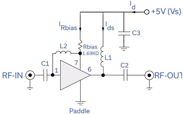
Fig 3. Recommended Application Circuit
