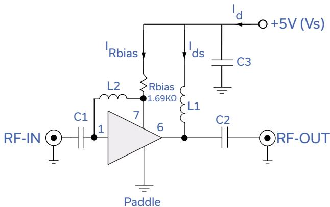
Fig 3. Recommended Application Circuit
