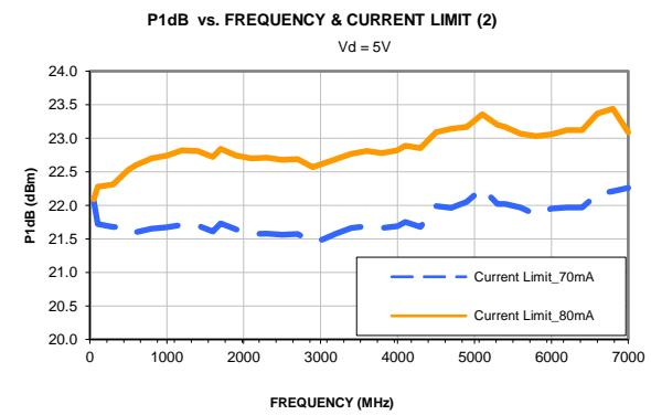
(1) External Rbias resistor is adjusted to obtain desired current
