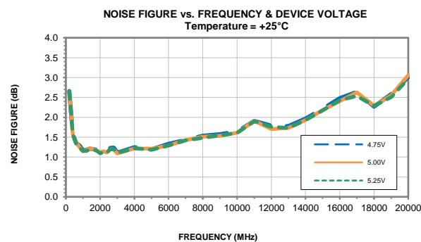
Note: Test data of Die packaged in industry standard 2x2 8-lead MCL package
