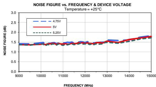
Note: Test data of Die packaged in industry standard 2x2 MCLP package
