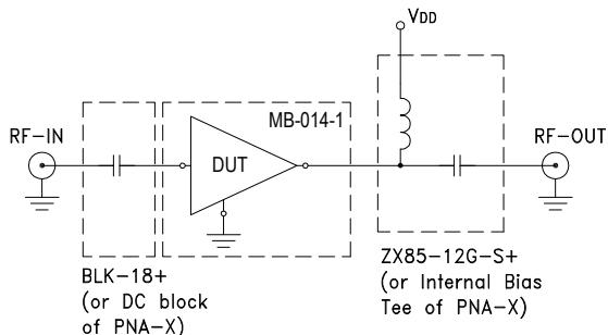
Fig 1. Characterization Circuit
