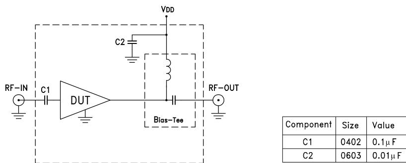
Fig 2. Application Circuit
