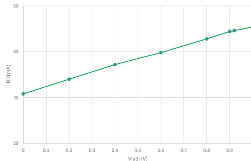
4. When Iadj connection is Open, Vladj=0.92V given a device with IDD=44 mA typ. For RF Performance at different Vladj, please see View Data and Graph.
