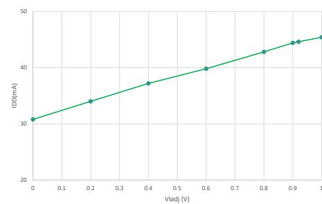
5. When ladj connection is open, V<sub>ladj</sub> = 0.92V given a device with IDD=44mA Typ. For RF performance at different V<sub>ladj</sub>, please see View Data and Graph
