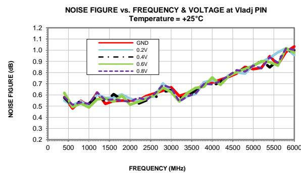
Note: Test data of Die packaged in industry standard 2x2mm 8-Lead MCL Package
