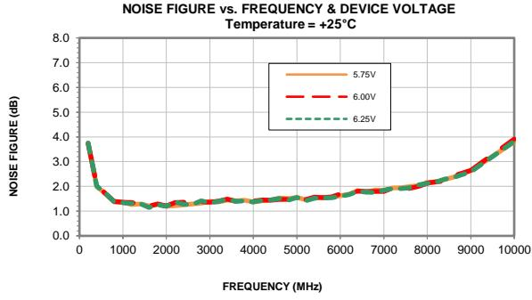
Note: Test data of Die packaged in industry standard 3x3MM 12-lead MCL package
