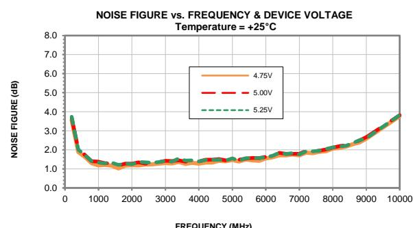
Note: Test data of Die packaged in industry standard 3x3MM 12-lead MCL package
