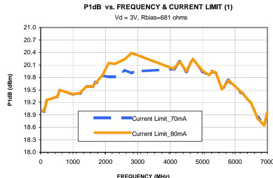
(1) Current is externally limited during P1dB measurements. Unit is capable of higher output power if current is not limited.
