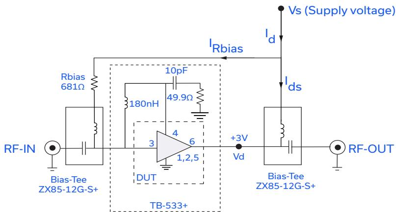
Fig 1. Block Diagram of Test Circuit used for characterization. (DUT soldered on Mini-Circuits Characterization Test Board TB-533+)
