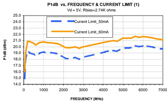
(1) Current is externally limited during P1dB measurements. Unit is capable of higher output power if current is not limited.
