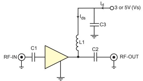
**Fig 2. Recommended Application Circuit**
