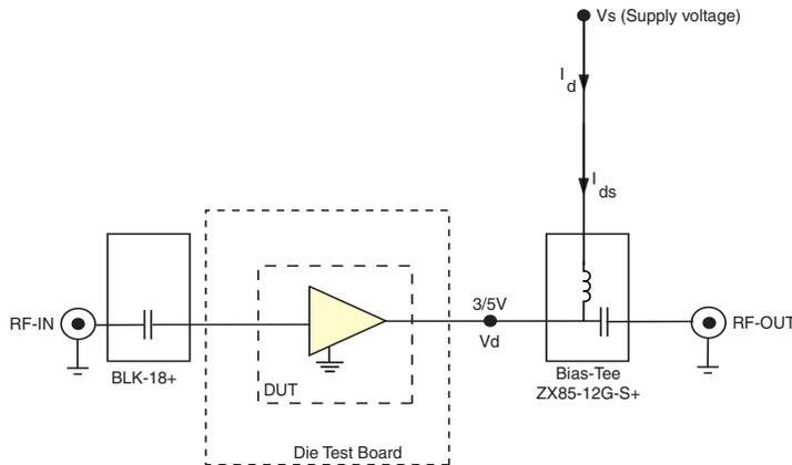
**Fig 1.** Block Diagram of Test Circuit used for characterization. Gain, Return loss, Output power at 1dB compression (P1 dB), Output IP3 (OIP3) and Noise Figure measured using Agilent’s N5242A PNA-X microwave network analyzer.
