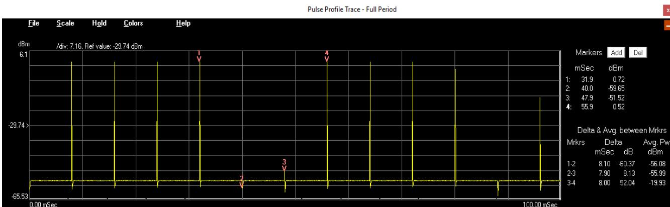
The main pulse profile display shows the full sample period of the sensor in the time domain.
