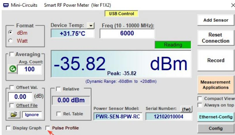
Enable pulse profiling and graphical pulse display, see page 8 for details.
