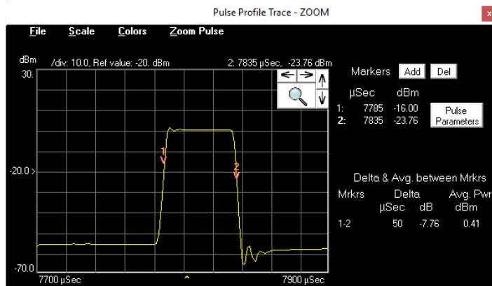
"Zoom on pulse" feature will automatically zoom on the first identified pulse and allows any portion of the pulse profile to be focused on / expanded in a second graphical display. Simply 'right-click' and drag the mouse cursor over relevant section of the profile.
