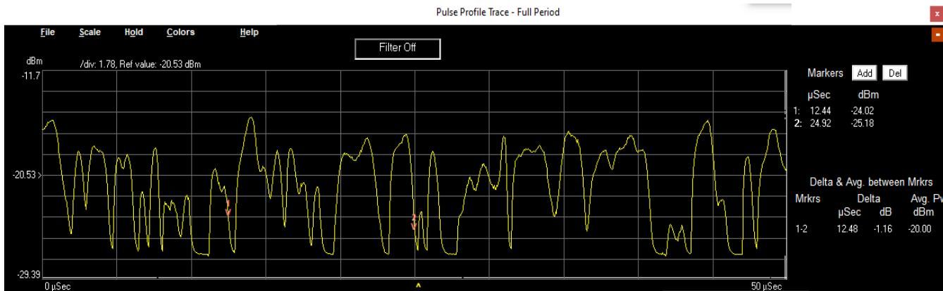
QAM256 in DECT setup, Gaussian filter @ 1.152 Msps
