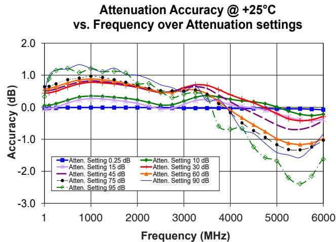
**Attenuation relative to Insertion Loss @ +25°C vs. Frequency over Attenuation settings**
