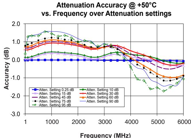
**Attenuation relative to Insertion Loss @ +50°C vs. Frequency over Attenuation settings**
