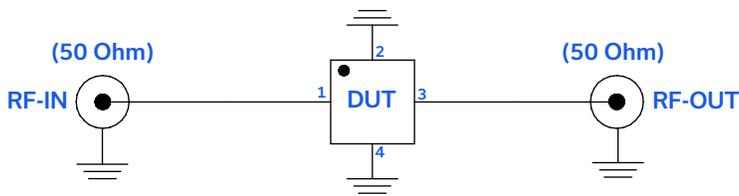
Fig 1. Block diagram of Test Circuit used for characterization. Characterization was performed by Modelithics, conditions test board details are available at: [www.modelithics.com/mvp/minicircuits](http://www.modelithics.com/mvp/minicircuits)
