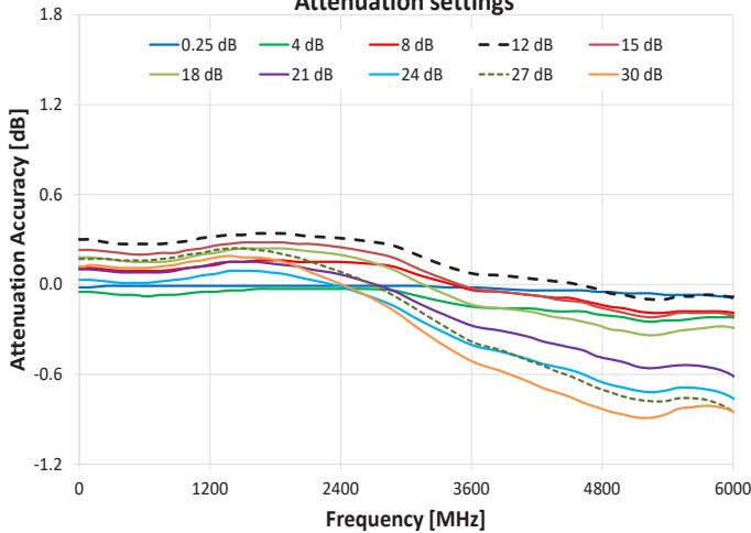
Attenuation Accuracy @ 50°C vs. Frequency over
