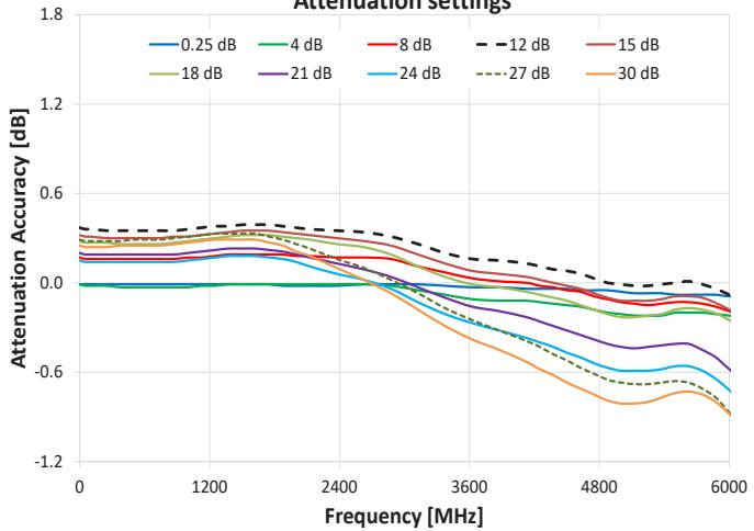
Attenuation Accuracy @ 1 - 6000 MHz vs. Attenuation
