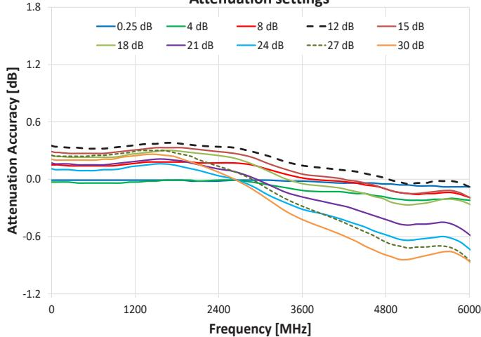
Attenuation Accuracy @ 0°C vs. Frequency over
