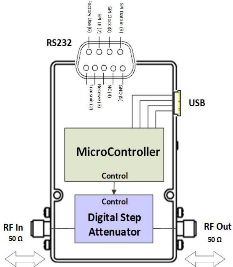
Simultaneous, bidirectional RF signal
