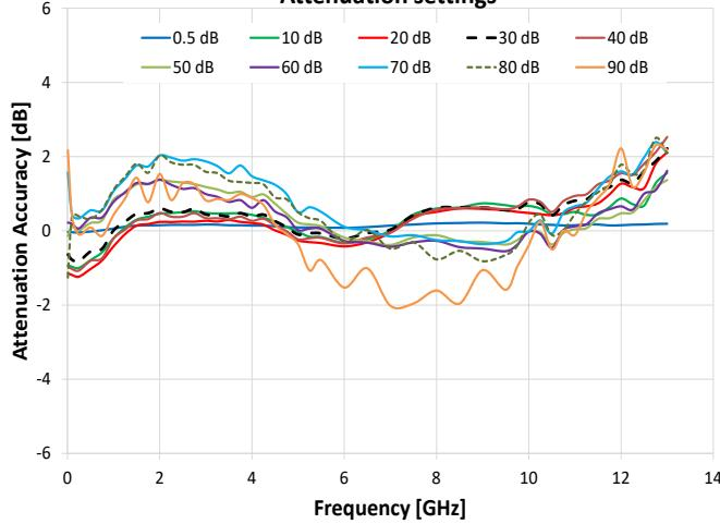
Attenuation Accuracy @ 50°C vs. Frequency over
