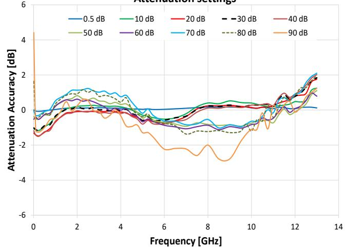
Attenuation Accuracy @ 0°C vs. Frequency over
