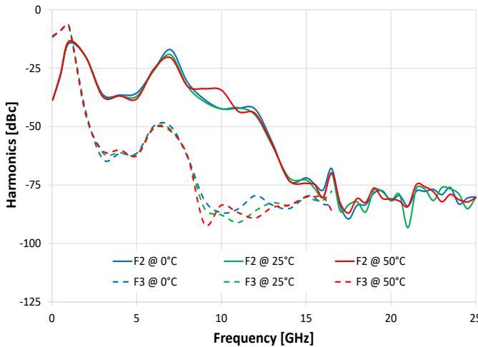
Sub-Harmonics vs. Output Frequency @ +10 dBm
