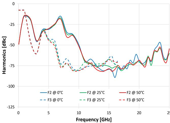
Sub-Harmonics vs. Output Frequency @ -20 dBm
