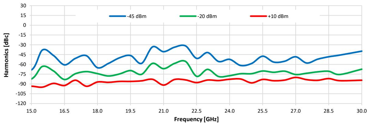
**Sub-Harmonics (F2.5) vs. Output Frequency**
