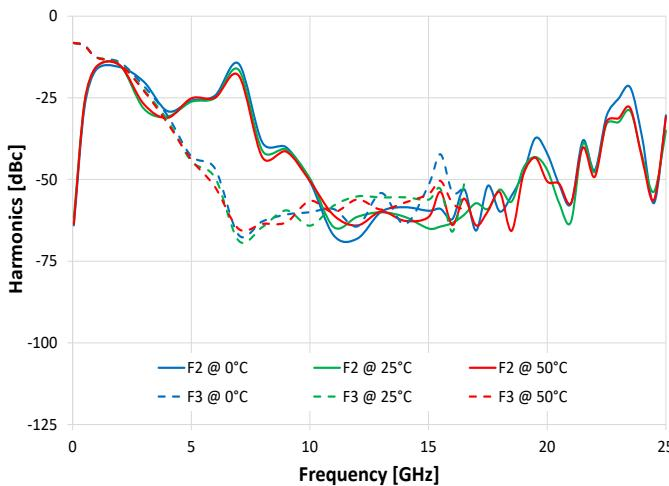
Sub-Harmonics vs. Output Frequency @ -45 dBm
