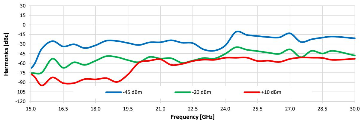
**Sub-Harmonics (F1.5) vs. Output Frequency**
