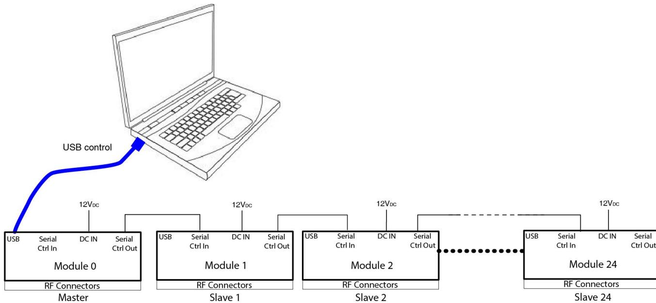
Connections between modules will be made using the serial in/out ports with the module connected to the PC act as a master and all other as slave modules. All control will be through the master module (address 0) which is the only one communicating with the PC or computer network. Serial control out port of each module should be connected to the serial control in port of the next module.
