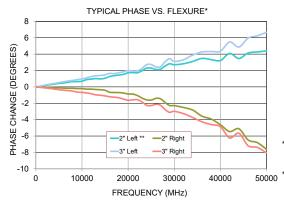
Typical phase change over flexure performed on T50-3FT-VFVM+ by wrapping cable 360° around 2" and 3" radii mandrels referenced to normalized straight position.
