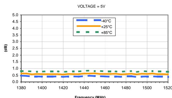
OUTPUT RETURN LOSS vs. FREQUENCY & TEMPERATURE
