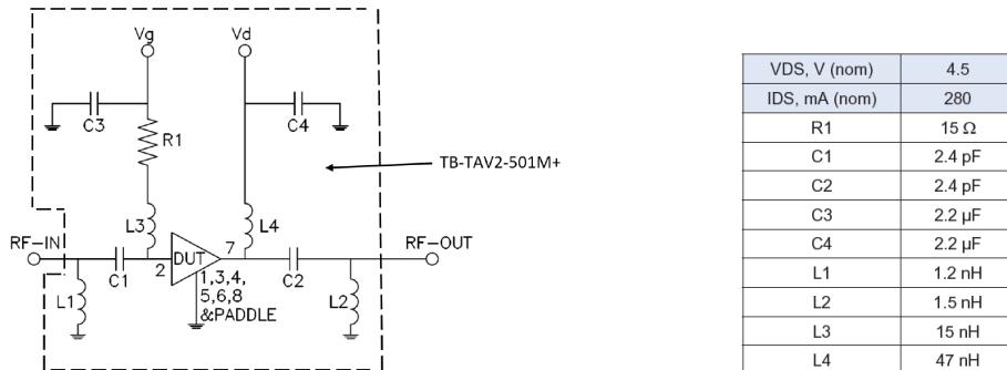
Fig 2. Recommended Application Circuit used for characterization. (Die is packaged in 2x2 mm, 8-lead MCLP package and soldered on Mini-Circuits Matching Circuit Test Board TB-TAV2-501M+)
