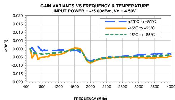
Note: Test data of Die packaged in industry standard 8-lead 2x2mm MCLP package
