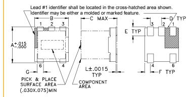
Pin 2 is not electrically connected. Solder attachment of Pin 2 is recommended for mechanical stability.
