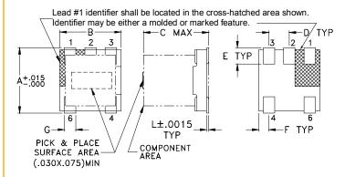
Pin 2 is not electrically connected. Solder attachment of Pin 2 is recommended for mechanical stability.
