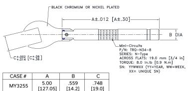
Dimensions are in inches [mm]. Tolerances: 3 Pl. ± .006 [0.150] Inch [mm] Torque Wrench Weight: 95 grams
