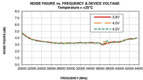
Note: Test data of Die packaged in industry standard 3x3 12-lead MCL package
