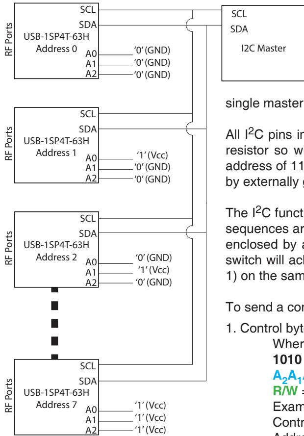
The I<sup>2</sup>C is a short-range synchronous communication protocol for simple 2-wire communication with slave devices using clock (SCL) and data (SDA) connections. The U2C-1SP4T-63VH interface also includes 3 address pins (A0, A1 and A2), allowing up to 8 switches to be controlled independently from a single master with shared SDA and SCL connections.
