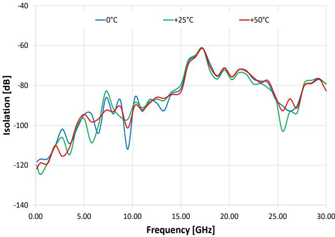
**Isolation J3 to J4 (J3 Active)**
