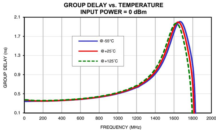
\* Temperature test data was based on the underlying chip.
