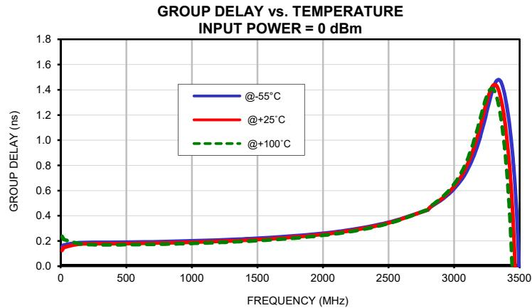
\*Temperature test data was based on the underlying chip.
