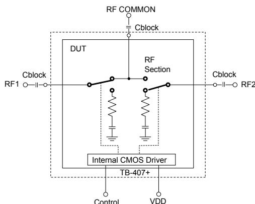
Figure 1: Block Diagram Of Test Circuit Used For Characterization.
