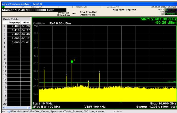
An application circuit was assembled to measure the IF reflection spectrum at the output of a mixer when the mixer was paired with a conventional filter versus a reflectionless filter.
