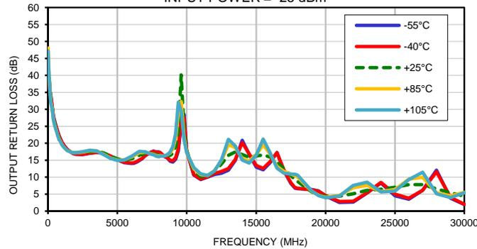
**OUTPUT RETURN LOSS vs. TEMPERATURE (Pass band)**
