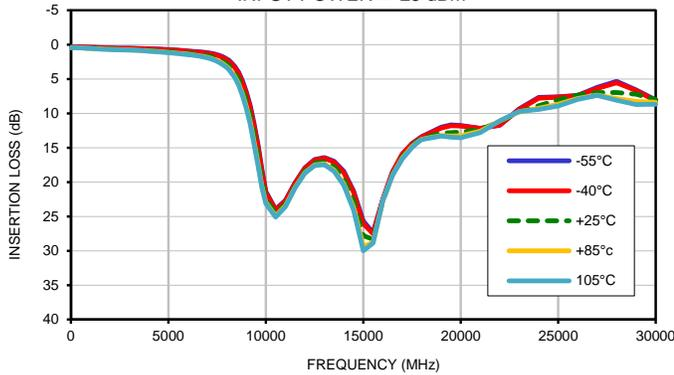
**INSERTION LOSS vs. TEMPERATURE (Pass band)**
