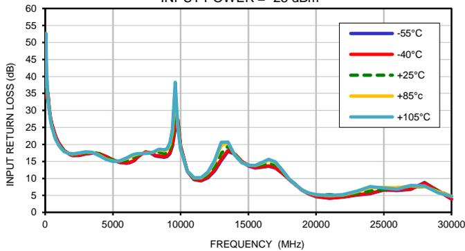
**INPUT RETURN LOSS vs. TEMPERATURE (Pass band)**
