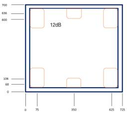
Fig 3. Bonding Pad Positions
