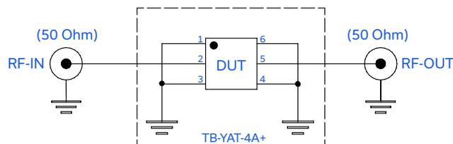
Fig 1. Block diagram of Test Circuit used for characterization, Test board TB-YAT-4A+ Conditions: Attenuation, VSWR: P<sub>IN</sub>=-10 dBm
