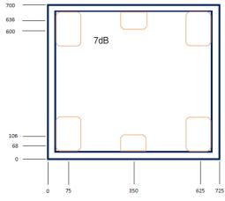
Fig 3. Bonding Pad Positions
